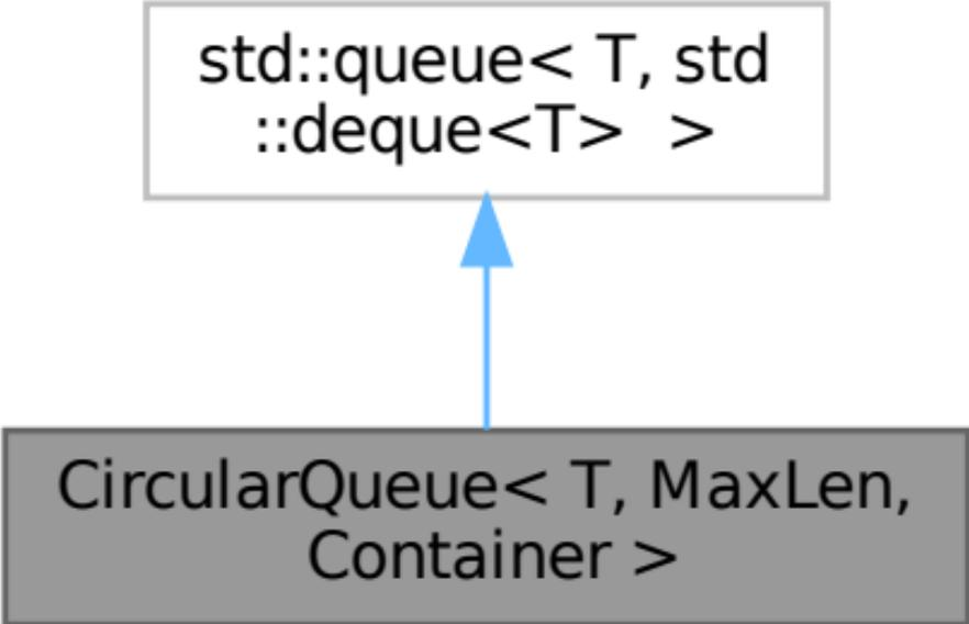
A diagram illustrating inheritance. A blue arrow points from the bottom box to the top box. The top box is white with a thin grey border and contains the text 'std::queue< T, std::deque<T> >'. The bottom box is grey with a thin black border and contains the text 'CircularQueue< T, MaxLen, Container >'. The arrow indicates that CircularQueue inherits from std::queue.
